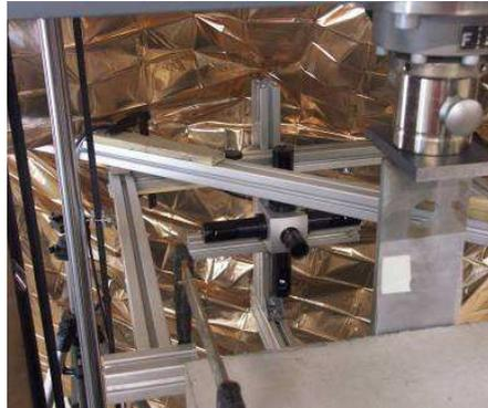
Fig. 4.1: Stiff connection between interferometer and concrete, shading to reduce outer light
