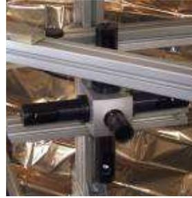
Fig. 3.2: Speckle interferometer with 4 reflector arms
